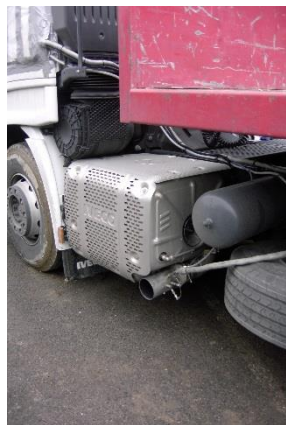
Exhaust Pitot flow meter, installed at the exit of the tailpipe
